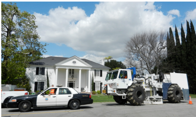
A two-phase, 3D seismic survey for Signal Hill Petroleum Inc. over and around Long Beach oil field involved seismic trucks sourcing in residential areas of Long Beach. Image courtesy of NodalSeismic.
