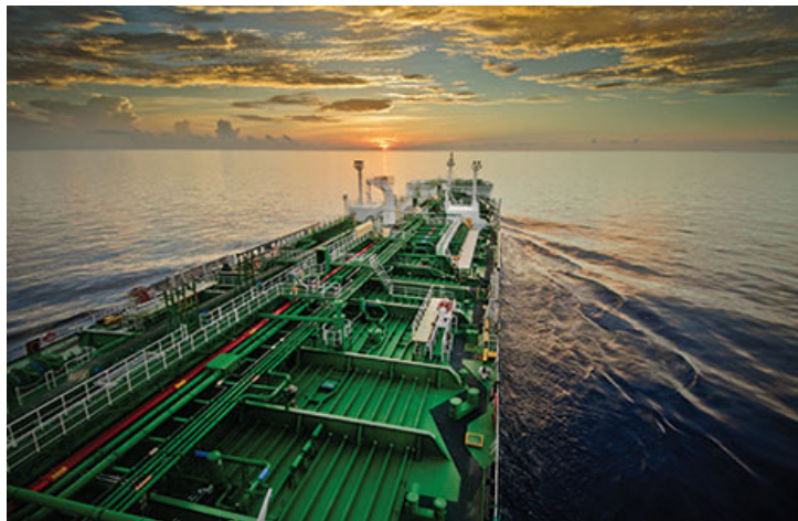
The MV Sunshine State is one of five state class, Jones Act tankers managed by Crowley for American Petroleum Tankers LLC. With an overall length of 600 feet and a beam of 105 feet, the vessel has a capacity to transport 332,000 barrels of petroleum products at a speed of 15 knots. (Photograph by Brian Gauvin)
